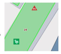
The NFPA standard symbol for shutoffs with "PV" for photovoltaic is utilized for Solar Panel Shutoff locations
